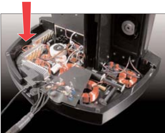
Figure 54. The location of the passive high-pass jumpers
