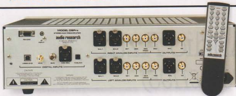
ABOVE: A choice of single-ended (RCA) and balanced (XLR) preamp outputs are joined by AES/EBU (XLR), S/PDIF (RCA, BNC and optical) and USB2.0 inputs. ARC's Soft/Sharp digital filter modes may only be changed via the partnering remote handset
