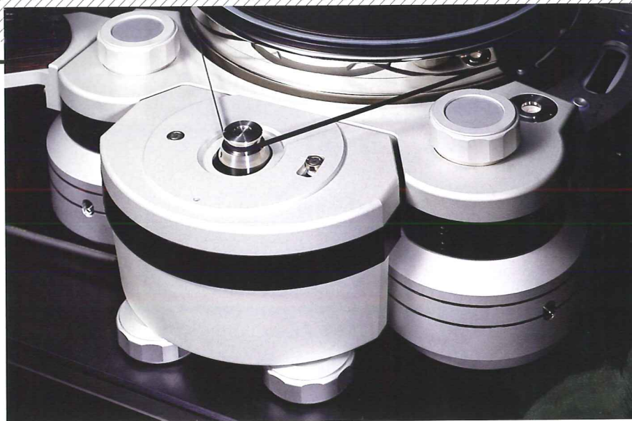
ABOVE: The huge AC synchronous motor is positioned adjacent to, but separate from, the main chassis. It is driven via a 2x50W amplifier for both phases and is adjustable in \pm 0.1 rpm steps
