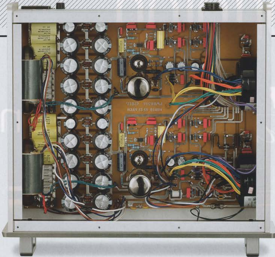
ABOVE: True dual-mono power supply features valve regulation, one 6H30 and one 6550WE per channel, with a couple of spares in the box. Two-channel topology extends to two connecting cables
